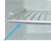
2b. Zip tie the advanced thermostat vertically to the underside of a net shelf in flat evaporator systems
